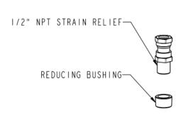
INSTALL REDUCING BUSHING INTO CASTING.
