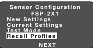
Recall Profiles allow the user to select the saved parameter profiles. This feature is used when programming multiple FSP-2X1s with the same parameters.
