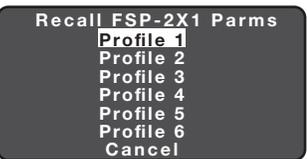
Selecting a specific profile allow the user to also change the parameters such as: High/Low Mode, Time Delay, Cut Off, Sensitivity, Setpoint and Ramp/Fade rates.
