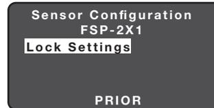
FSP-2X1 default settings communicate with the FSIR-100; however, this security feature limits communication only for authorized installers who have access to main power supply to the FSP-2X1 sensor. Press Select to set Lock Delay or press PRIOR to go back.
