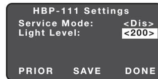
Presents light level to the HBP-111. The light level reading can be used as a reference for setpoint adjustments.
