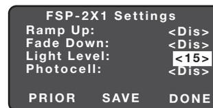
Displays the light level at the FSP-2X1. The light level reading can be used as a reference for setpoint adjustments.
