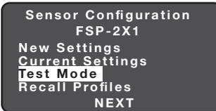
Test Mode shortens timeouts for High/Low and Cut Off, to allow quick verification of settings. Test Mode disables automatically after 5 minutes.
