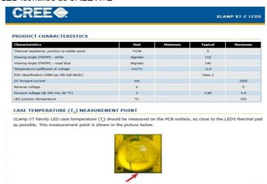
Maximum Junction Temperature from LED specification (Tj) =  $150^{\circ}$  Thermal Resistance Formula from LED specification =  $5^{\circ}$ C/W Maximum Forward Voltage (Vf) from LED specification = 3.4V Measured LED Current = 305mA Calculated LED Wattage = Vf x Measured LED Current = 1.037W Maximum Source Temperature (Ts) = Tj – (LED Wattage x Thermal Resistance) =  $144.8^{\circ}$ C
