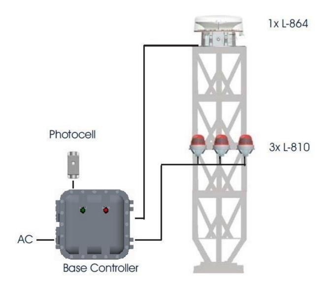
Figure 2 - Typical System A1 Connection Configuration
