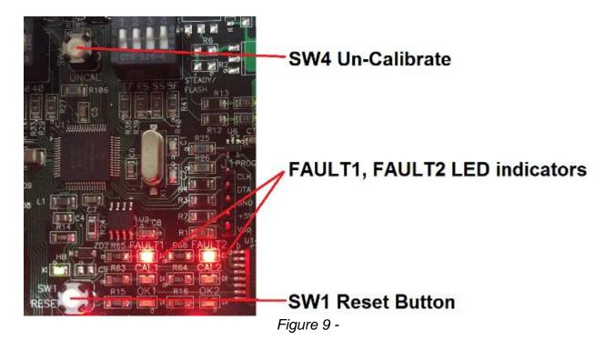
Note that a correct calibration will have a green LED lit labeled OK1 if there is a connection detected at Port 1, and a green LED lit labeled OK2 if there is a connection detected at Port 2. A red FAULT LED followed by an alarm will indicate that there are two or more L810 lights not functioning or if port is being utilized for an L864 beacon, the beacon is not functioning.
