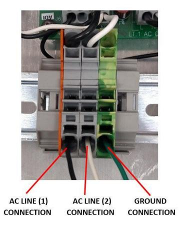
Figure 6 - AC Wire Connections
