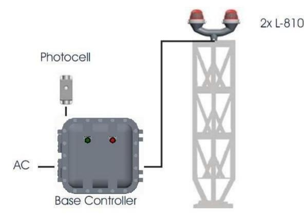
Figure 1 - Typical System A0 Connection Configuration
