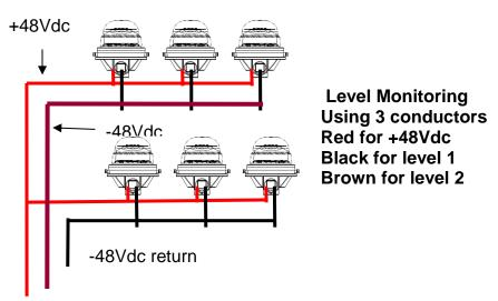
Level monitoring using 3 conductors allows for the system to know what level the fault is on but visual inspection is required to verify which light is faulty.
