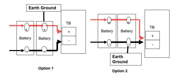
**NOTE:** Additional Earth ground may be included in the installation process and **MUST** be connected to the Aluminum plate located inside the enclosure.
