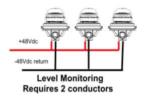
Level monitoring **does** require visual inspection for a single faulty light. The controller will indicate an event plus a LED AL7 will illuminate for a faulty light.
