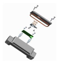
Open supplied photocell enclosure. The Photocell requires 3 connections to be made to the inside of the photocell enclosure itself and 3 inside the controller.
