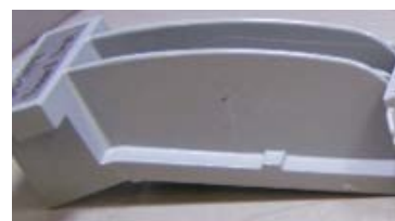
Dialight product after 3000-hour Salt Spray Testing (ASTM B117)
