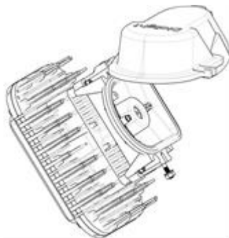
Figure 10 - Hang Light Fixture onto Stanchion Mount
