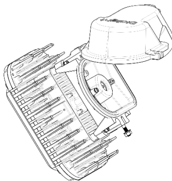
Figure 3: Hang Area Light onto Stanchion Mount
