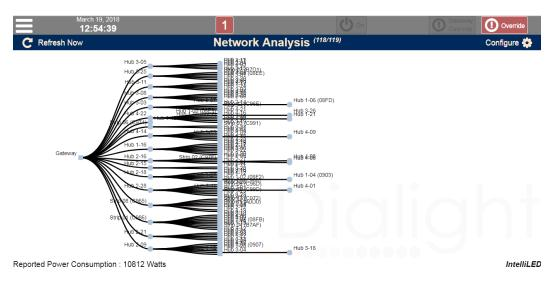
The Net Analysis page shows a graphical representation of the tree formed by the wireless mesh network that is used to control the lights. This is useful in understanding the network connectivity and general health of the wireless network. This is helpful for troubleshooting issues on site.
