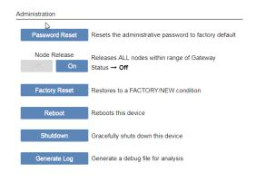
NOTE: Node release will go through a 'transition' phase inbetween On/Off. This can take up to 1 minute
