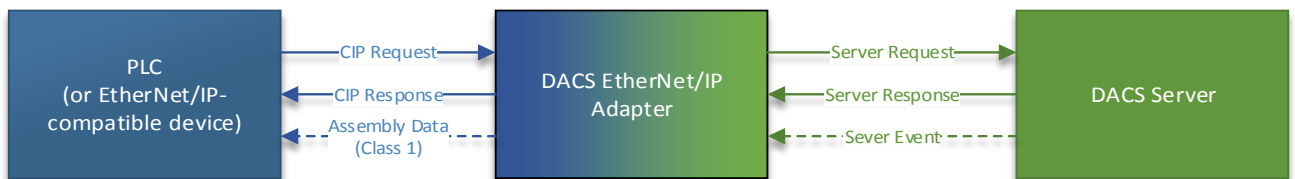
Figure 1- Communication between PLC and IntelliLED server
