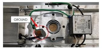
2. Remove the 2x 6-32 Philips SEMS screws and remove the surge module from the luminaire (shown below). Discard.
