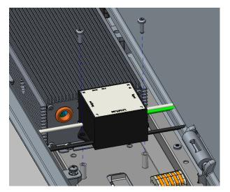
3. Install the new surge module using the supplied 2x 6-32 Philips SEMS screws (shown above). Torque to 12-15 in-lbs.
