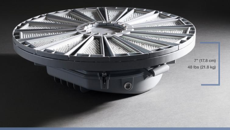
This state-of-the-art fixture builds upon the performance of our popular High Output High Bay series with a lighter, lower profile design offering greater ease of installation. At just under 7" (17.8 cm) tall and 48 lbs (21.8 kg) this powerhouse can reach up to 71,000 lumens for mounting heights up to 100' (30.5 meters).
