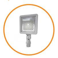
Mount to 2" round poles (2-3/8" OD) Integrated Slipfitter has locking positions from 0°-180°, in 7.5° increments Gasketed wiring compartment
