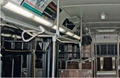
White LED lights for fluorescent replacement provide significant maintenance savings for US Transit Buses.
