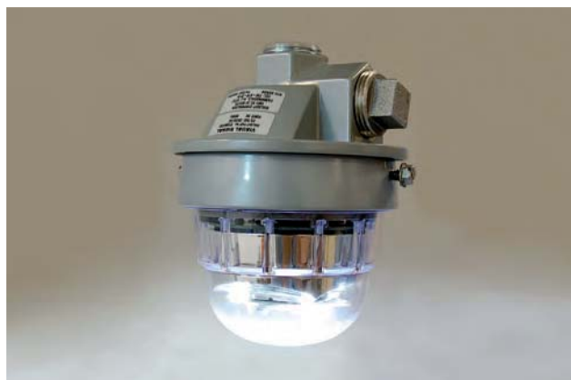
Introduced as a highly efficient alternative to incandescent "jelly-jar" fixtures commonly used in industrial and hazardous locations, the SafeSite® White RTO consumes just 8 watts. The products are certified to meet UL1598 and UL 844 Class I Division 2 requirements.
