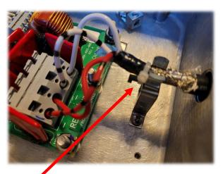
Insert braiding in to the clip and use zip tie to secure to clip. See NOTICE on inside lid of flashhead for more details.
