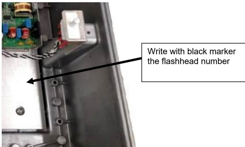
4. The Flashhead RED cables braiding must be fed under each of the Grounding clamps and **secured tightly**. The BRAID of the cable must be in contact with both the panel and the grounding clamps and then secured under the clamp.
