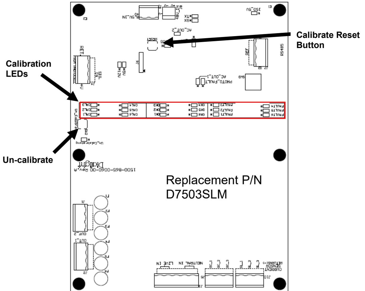
If no side lights are being installed then the installer should still calibrate to zero out the calibration. Re-calibration is required whenever a Side light is added or when a Side light is replaced.
