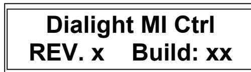
**NOTE:** The Site Manager and Installer should take note of this screen including the REV number and the Build number if any future troubleshooting is required. x’s indicate revision levels and will appear as numbers on the display.
