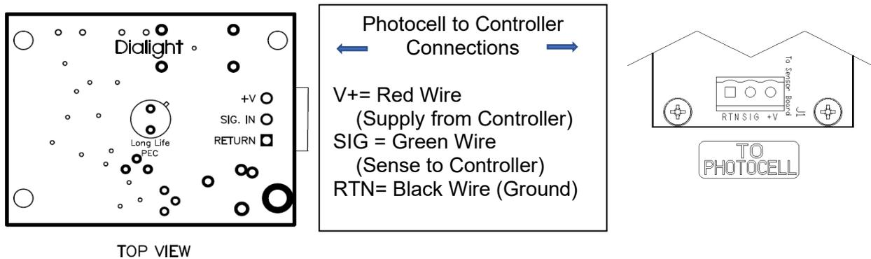
**NOTE:** A zip tie is provided inside the photocell enclosure to secure the cable from falling out. A UL knot can also be used to prevent the cable from sliding down the conduit. Weight of cable should not be placed on terminal block alone.
