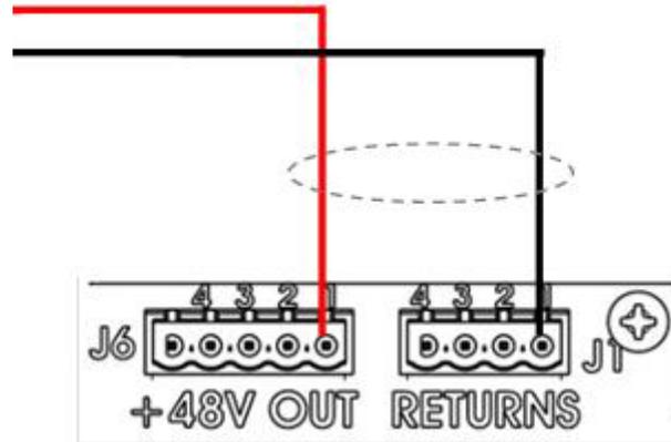
Connect the sidelight wires, if applicable, to the Marker Light Monitor Board in the Controller as shown in the diagram above. Connections are made to J6 (+48V OUT) and J1 (RETURNS) of the Marker Light Monitor Board. Connections must be made on the same pins at J1 & J6 (1-1, 2-2, 3-3 or 4-4).
