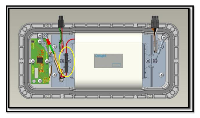
3. Unscrew the two M4x.7 screws to remove the pack and save the screws to assemble the replacement battery pack. Discard old battery pack according to respective national regulations on waste disposal.
