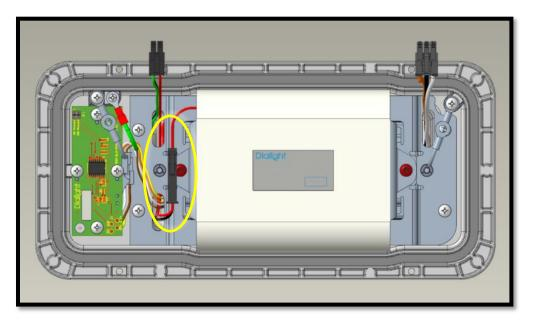
6. Optional Step - If required, on the Runtime Board as displayed in the images below, the jumper can be toggled between 60- and 180-minute positions as highlighted to change the operational time of the light on Battery Backup mode and if the jumper is not used then it will default to 90 minutes. (NOTE: FOR UL924 APPLICATIONS, 60 MINUTE DURATION MUST NOT BE SELECTED)
